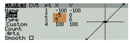
You can also add extra points between p1 and p4, for example to set a non-linear response, and/or to limit the snapflap at a certain point in the elevator travel.
