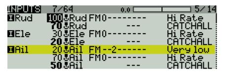
*Safety note:* the last input line in a group should act as the default, with all flight modes checked (the 'CATCHALL' lines in the example above).
