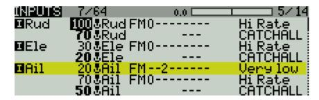
Safety note: the last input line in a group should act as the default, with all flight modes checked (the 'CATCHALL' lines in the example above).
