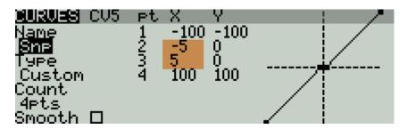
You can also add extra points between p1 and p4, for example to set a non-linear response, and/or to limit the snapflap at a certain point in the elevator travel.
